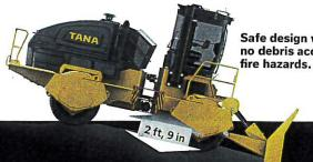
Safe design without belly pans: no debris accumulation to cause any fire hazards.
